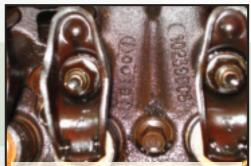
The top of the head reveals the rockers and valve springs have almost no deposits. Note the part numbers still are visible.
