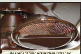
The engine oil pump pickup screen is very clean and has no deposits.
