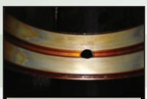
The upper main bearing shows very little wear. All of the main bearings from the engine are in useable condition, according to the analysis.
