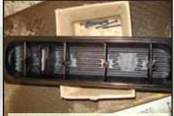
The inside of the valve cover is very clean with almost no deposits.
