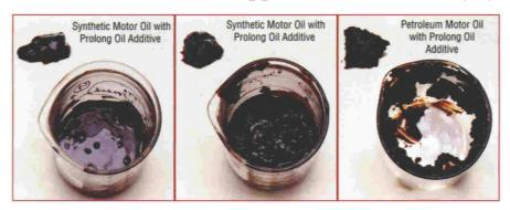
Oil Analyzers Inc. (OAI) has recently performed oxidation testing on samples of new motor oil treated with chlorinated aftermarket oil additives and compared the results to oxidation testing of untreated new motor oil in an effort to determine the cause of severe sludging in the field. The treated samples produced gels (shown at left). Unadditized motor oils do not. The gels appear to lead to sludge formation.
