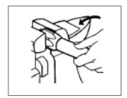
Place socket in vice and screw in hose counter-clockwise until hose bottoms. Back hose out ½ turn.
